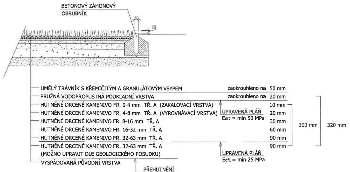
POZNÁMKA: ZAKALOVACÍ VRSTVU PROVÉST RUČNĚ V MOCNOSTI 5 mm (MAX 10 mm)
