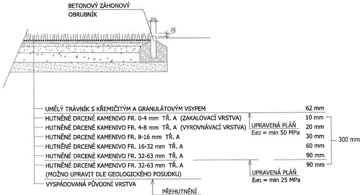
POZNÁMKA: ZAKALOVACÍ VRSTVU PROVÉST RUČNĚ V MOCNOSTI 5 mm (MAX 10 mm)
